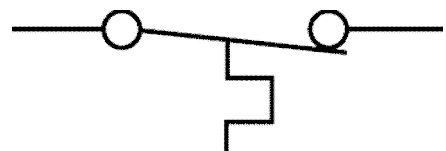
SPST Opens on Drop (Safety Control)
