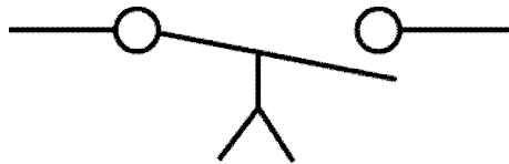
Time Delay Relay Delays Closing (Mechanical/Thermal) (Electronic)
